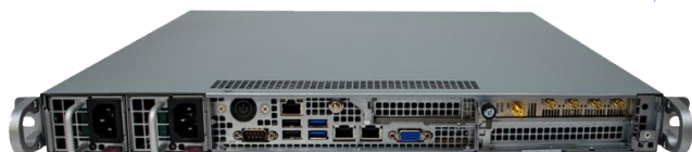
The Monics 1500 sensor provides frequency and advanced time domain measurements.
