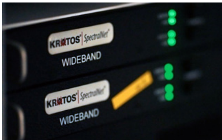
SpectralNet Wideband digitizers at Kacific gateways convert RF signals into IP packets to remove distance barriers in RF signal transport. Source: Kratos
