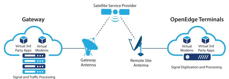
The OpenSpace Platform is an end-to-end digital satcom system from the gateway to the OpenEdge remote.
